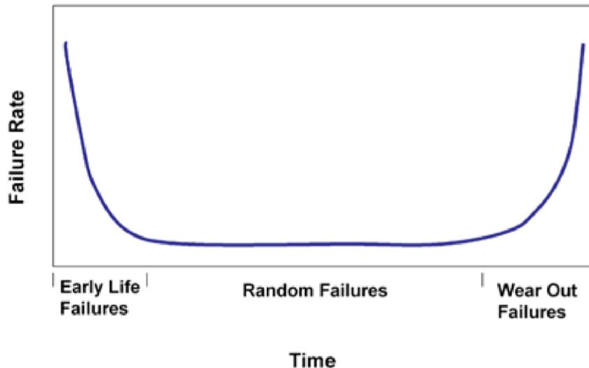
Several speakers displayed charts like the one above. The chart has three distinct areas. It applies to modules and inverters. Interpreted for modules, cell cracks are the failure dominating in the first two years, PID by shunts in 3-4 years. The failure rate then stays low for a few years. Discoloration occurs over time and causes modules to fail after about 18 years, a time when failure rates return to a high level.
